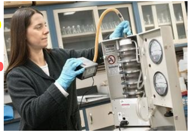
Clarkson University Professor of Civil and Environmental Engineering Andrea Ferro with a MOUDI cascade impactor, an instrument that separates and collects airborne particles in nine size ranges from 0.18 mm (micrometer) to 18 mm, which she uses in her research on indoor air pollution. Here, she checks the flow rate through the MOUDI using a Bios electronic flowmeter. Particle size is important in Ferro's research because the size of a particle affects where in the respiratory tract it will deposit. (Photo courtesy of Clarkson University)
